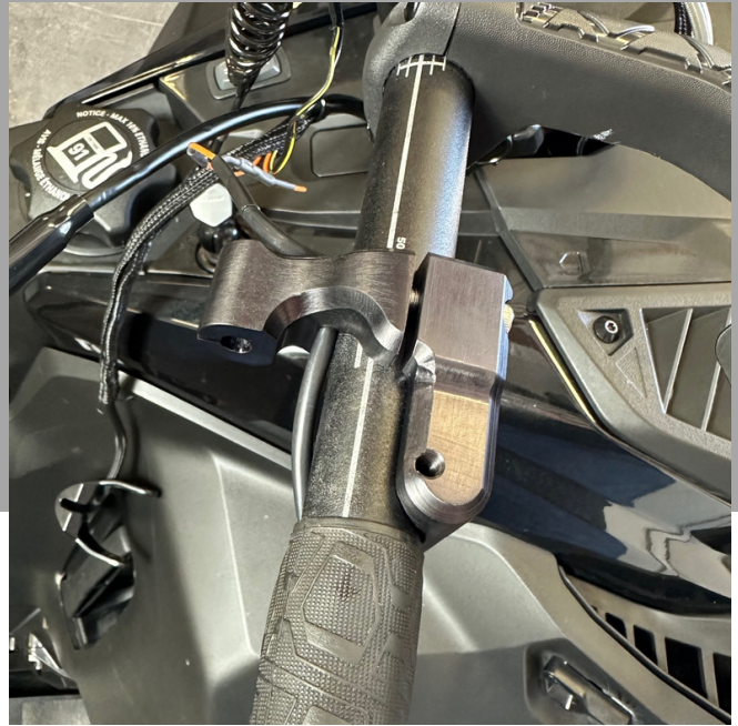
14. Install new Force Turbos Throttle Block. Make sure logo is facing forward and hand warmer wire is placed on the back side. Adjust to comfort level.
