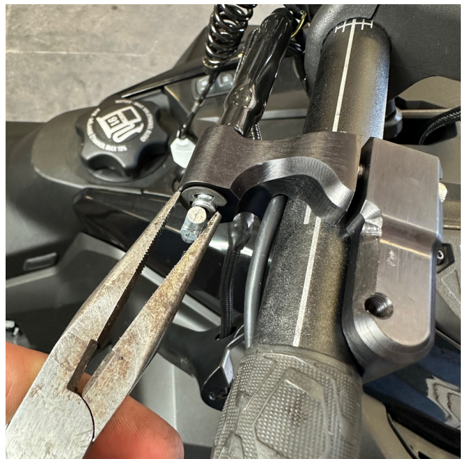
16. Re-install the c-clip that was removed in step 5.
