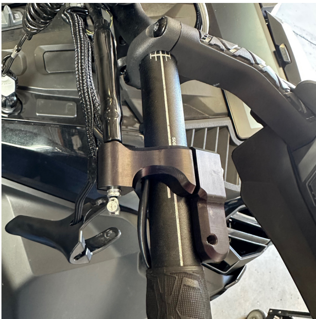
15. Use needle nose pliers to pull throttle cable through the wire groove of the throttle block.
