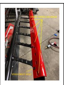
**Figure 2.** Stock tread lug holes and stock rivet hole.
