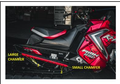
**Figure 1.** There is one left and one right Ultimate Edge rail cap. The small chamfer and group of two weight reduction holes should be at the front of the sled.
