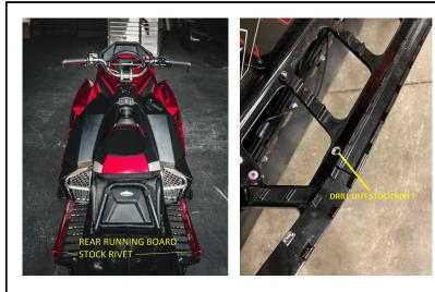
Figure 3. Stock rivets.
