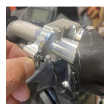
10. Remove the c-clip from the pivot pin on the throttle flipper. Be careful not to lose this.
