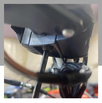
8. Loosen the 5/32 allen stud from the bottom of the throttle block.
