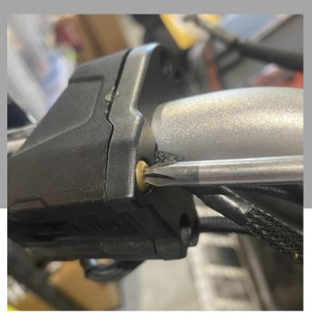
9. Remove 4) gold Philips head screws from the side of the throttle block. Slide the cover back and off the handlebar.
