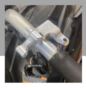
19. Install your new Force Turbos throttle block with provided bolts. Make sure to put the wires in the slot without pinching them.
