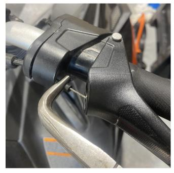
11. Remove the cable from the throttle trigger. (Pull it to full throttle position. Gently squeeze with needle nose pliers. Put back to zero throttle position. Remove T-crimp).
