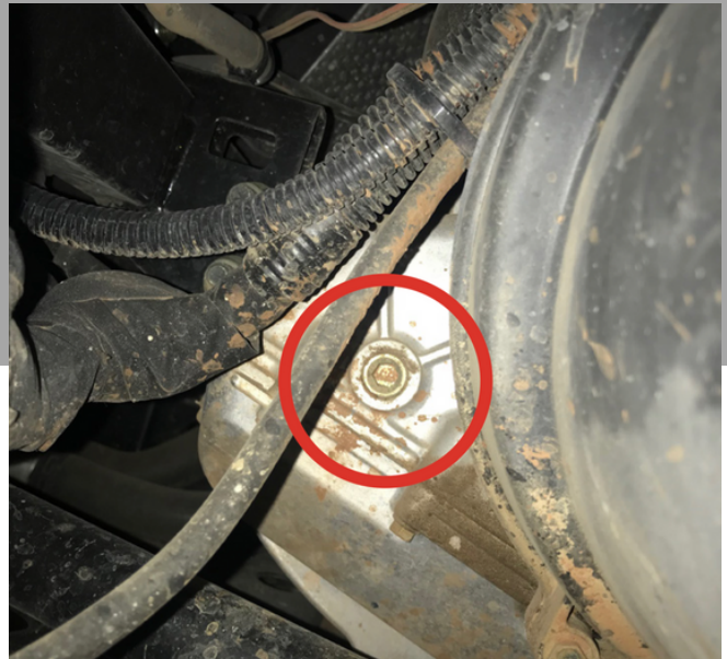
8. Find and remove drain plug on the driver's side in front of clutches
