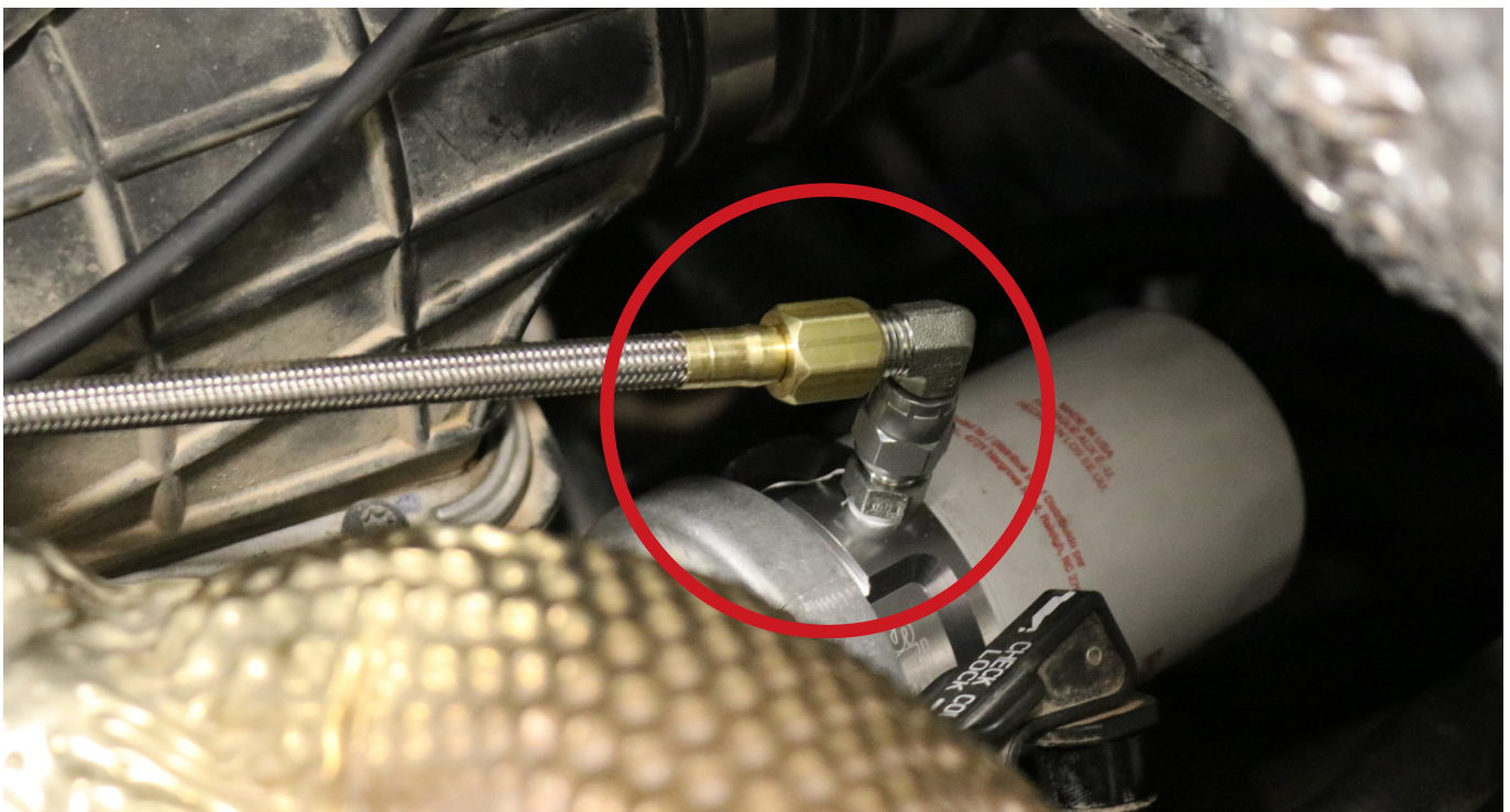
15. Install oil line from turbo to sandwich plate
