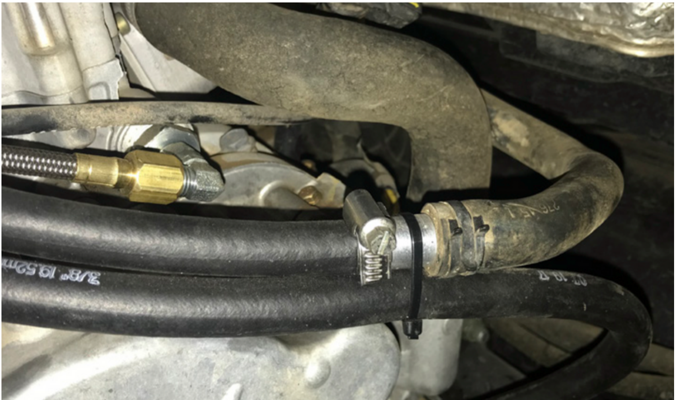
13. Run coolant line to the back of the vehicle and zip tie lines away from exhaust
