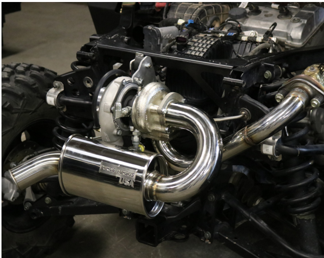
5. Mount turbo system. Install rubber mounts first, line up the exhaust flange, and install the two exhaust bolts and springs. Next, install nuts on the rubber mounting studs, line up your bracket mount, and install nut and bolt
