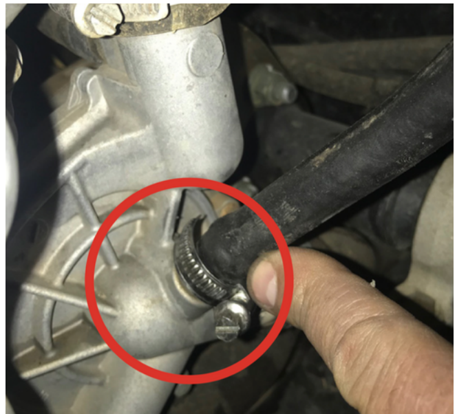
10. Remove coolant line from water pump under right hand throttle body and cut off first 90° section in stock line
