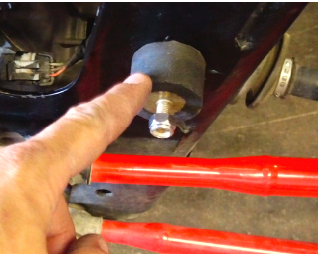
9. Drill out frame holes on the lower frame to 3/8", making them ready to accept rubber mounts
