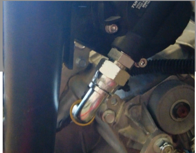
8. Ensure that the pump is not touching the frame after installation. The pump flow arrow should be pointing upwards
