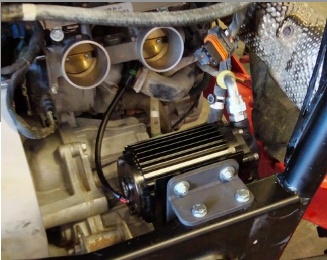
7. Bolt scavenge pump to frame using 13mm bolts
