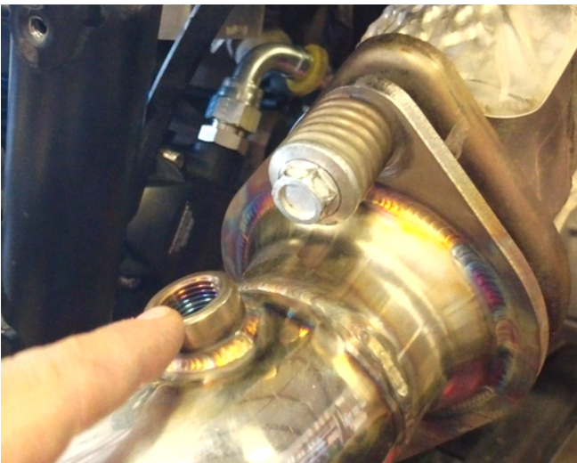
16. Install the stock O2 sensor onto the turbo inlet pipe just after the manifold connection
