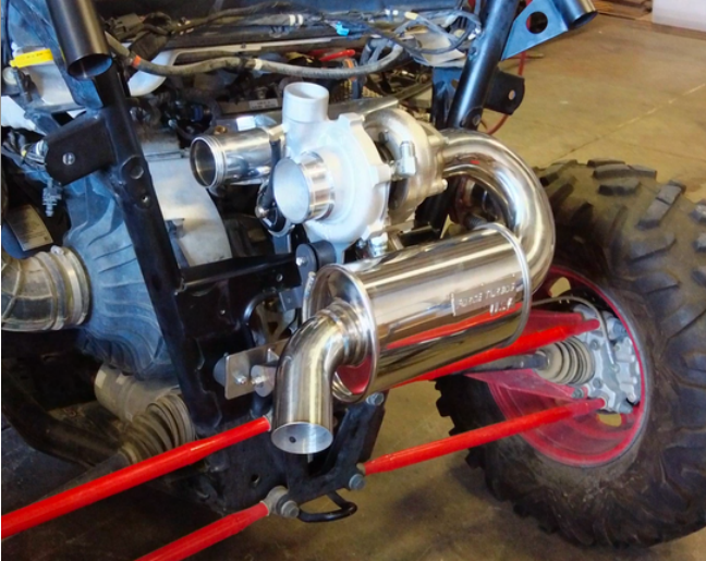
14. Install the turbo onto the lower rubber mounts. Install the spark arrestor
