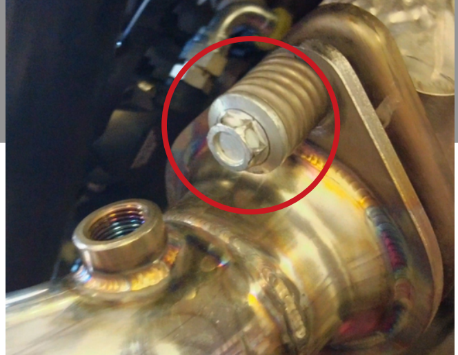
15. Attach the right side of turbo to the machine with stock bolts and springs
