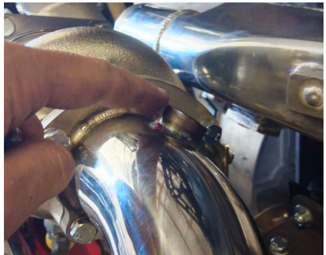
17. Install the AFR sensor for the Dynojet into the exhaust just after the turbo
