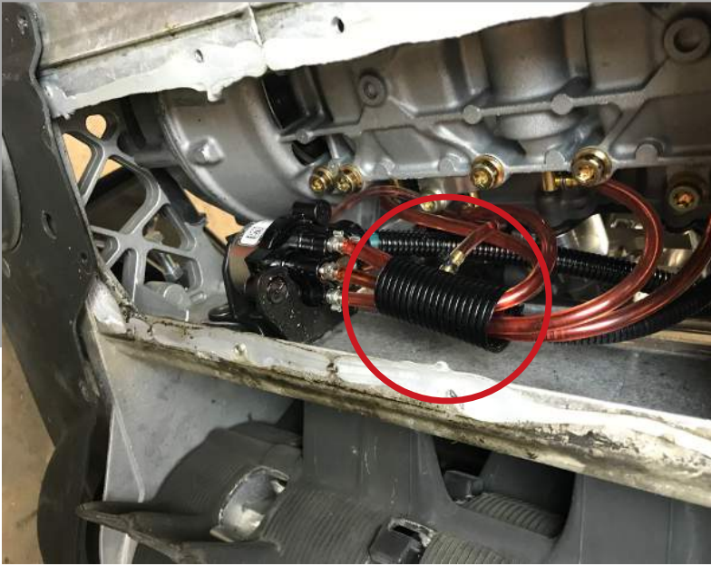
15. Reinstall oil line wear covers on oil line. Reinstall access panel and rivet back into place
