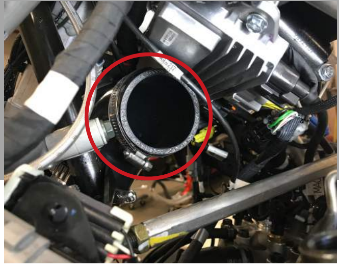
20. Install the 3" silicone 90 onto the double inlet airbox. Point 90 to the right hand side of the vehicle. Make sure that the constant tension clamp will not run on the PBR voltage regulator when install is finished
