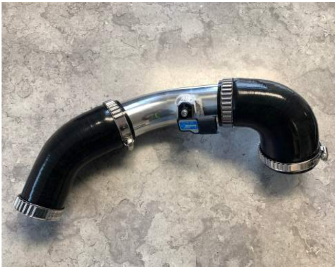
21. Install 3 bar map sensor into the charge tube. Connect snowmobile map sensor wiring to the new 3 bar map sensor
