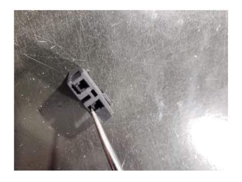
13. Install both terminals into the new connector housing. Plug the mating connector on the pump assembly together making sure everything fits properly.
