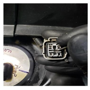
16. Using the pick remove the terminals from the connector housing. The same style tab holds the terminals in the housing.
