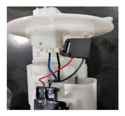
12. Insert the terminals into the new connector provided. Red to red, black to black. The new connector has the same tab holding in the terminals if you need to remove it. You should hear a click on the terminal once installed correctly. Do not force the terminals in the housing. They only go one way.
