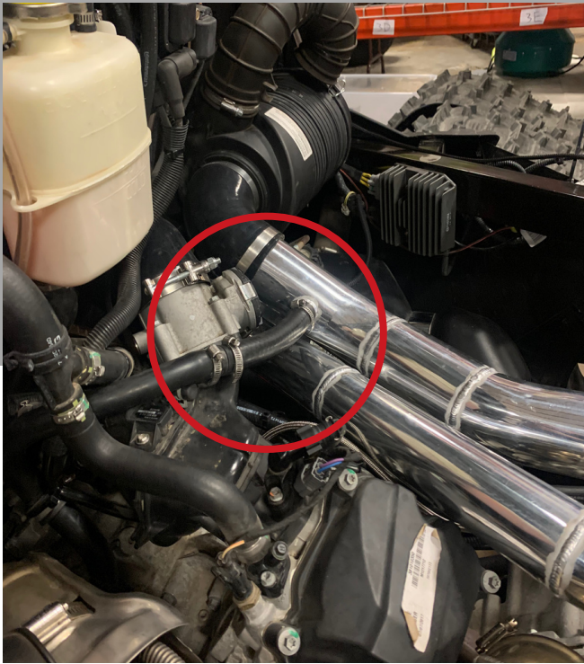
21. Connect crank case breather line to 3" turbo cold air intake
