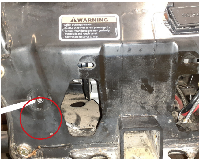
9. Bolt turbo exhaust muffler back onto turbo loosely. Mark mounting hole for rubber stud mount. Remove turbo exhaust muffler. Use 21/64" drill bit to drill hole where rubber studs will be mounted (when drilling, make sure you do not hit transmission with drill bit). Mount rubber stud into hole
