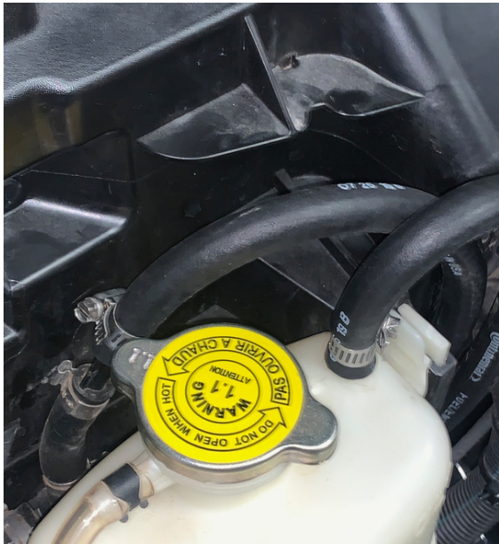
16. Install coolant line on Y fitting and run to rear side of the turbo. Install second coolant line on top of the coolant bottle and run to front side of turbo. Feel free to trim coolant lines if needed. Zip-tie coolant lines out and out of the way of moving parts or shifter linkage.
