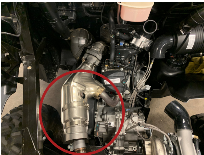
8. Tighten exhaust clamp and reinstall exhaust heat shielding. Reinstall stock O2 sensor and plug in
