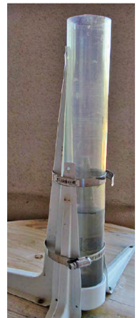
Figure 6: Test stand for measuring evaporation of water at different conditions
