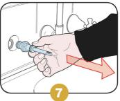
Remove the spindle. Ensure that washer is removed and the tap seat is clean
