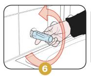
Using the tube spanner, loosen the spindle
