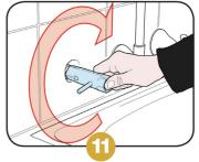
Using the tube spanner, tighten down the lock nut. Turn on the water to make sure there are no drips at the base. Tighten the spindle if it is dripping.
