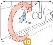
Using adjustable spanner on the brass flat spots, tighten the XValve
