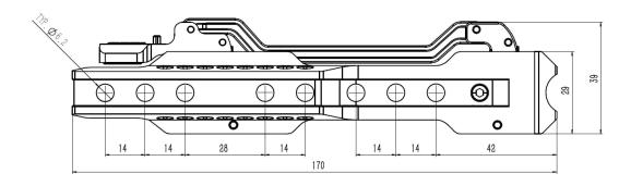
**Note:** Use M6 screws to fix the mount on the riflescopes.
