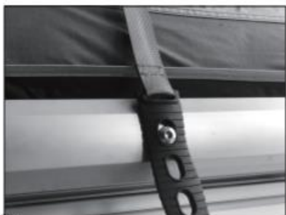
⑤ Keep pulling the webbing till you get the adjustable rubber hook.
