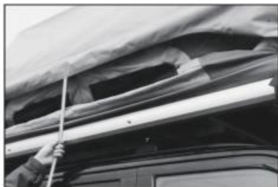
④ Close the roof tent by pulling the webbing.
