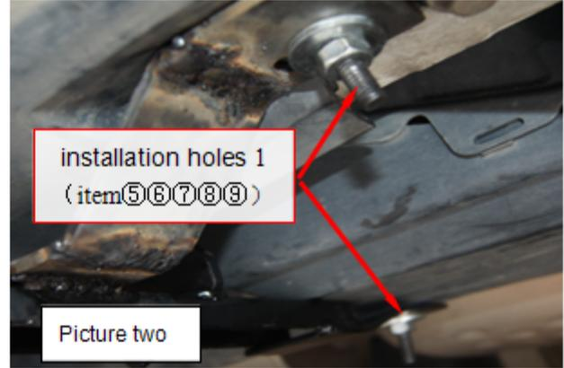
Step Four: Install Left rear brackets, referring to picture two. Put the ⑧ (φ8 plastic block) mounted to ⑨ (T bolt ), put part number ⑨ into the two hole positions, reuse parts ⑤⑥⑦ of the chassis pieces, don't tighten the bolts yet (the left and right bracket are fitted in the same way)
