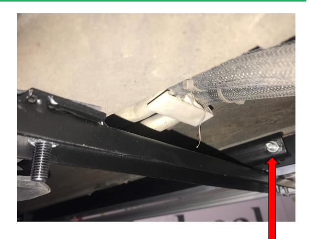
Place the bracket at the front of the sill then put the clamp in place over the lip of the sill to securely fit in place.
