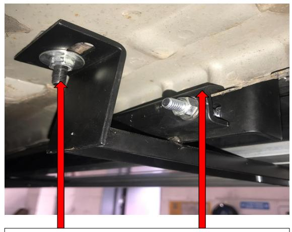
Remove the bung in the chassis on the off side at the rear of the vehicle, again place the T-bolt into the hole in the chassis and the welded part of the bracket at the front of the sill, clamp along the lip on the sill using the bracket provided to hold firmly in place.
