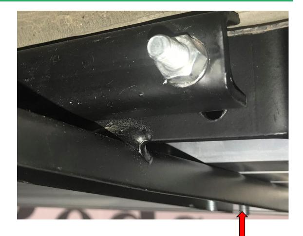
Once the brackets are in place slide the bolts along the side steps to fit each step. Place at 45 degrees to make sure rubber goes to the back of the sill, press down and firmly fix in place on each bracket.
