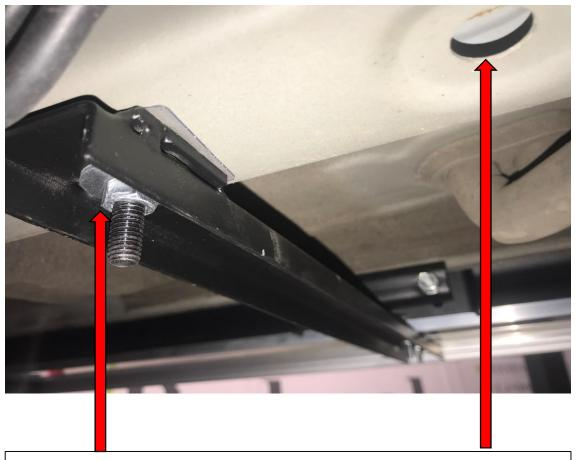
To fit the bracket, place the T-bolt in the hole in the chassis. There are a number of these along the car chassis on the nearside.
