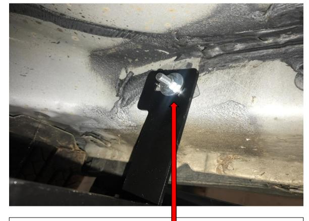
On the front fixing part of the bracket you may need to remove some of the sealant to reveal the hole for the front part to fix to, then place a 6mm T-bolt in this hole. Use the plastic washer to stop this falling into the channel and fix in place.
