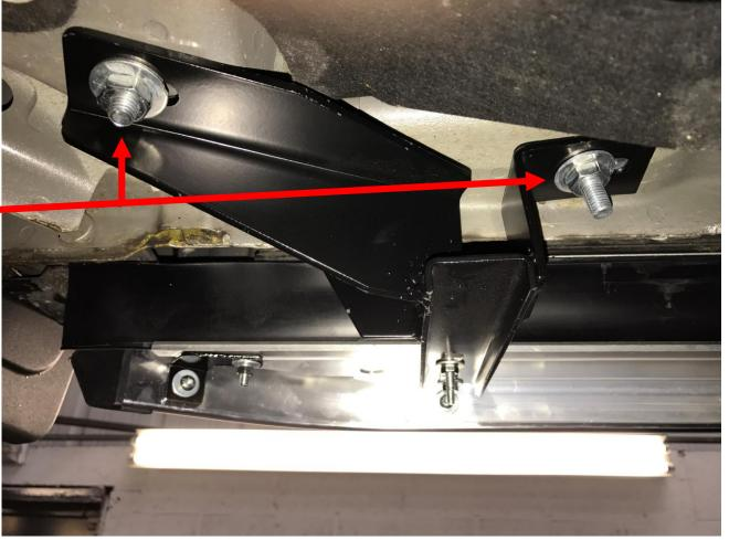
The is also a hole is the sill that you will need to use for the bracket. The Small T-Bolt sits in this hole.
