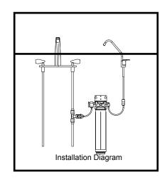
7. Locate the cold water pipe you will tap into to supply water to the filter system. DO NOT USE THE HOT WATER PIPE. Turn off the water to the cold water feed pipe. Attach (A) self piercing saddle valve to the cold water pipe per instructions included within the valve packaging ensuring you have adequate room to connect the 1/4" tubing. Attach connector (B) to the saddle valve and insert 1/4" tubing (C).
