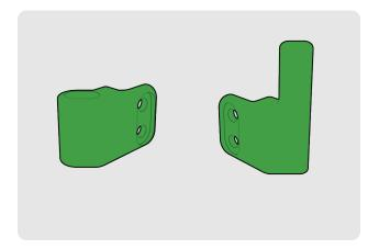
Screw these edge connectors into the new side door panel in the orientation shown below. Be sure to pay extra attention to both the orientation of the connectors and the orientation of the panel.
