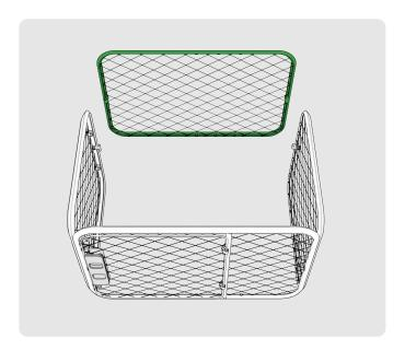
On the new side door, remove the edge connectors using a phillips head screwdriver. We recommend opening the door to allow better access.
