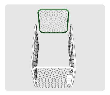
On the new door, remove the edge connectors using a phillips head screwdriver. We recommend opening the door to allow better access.
