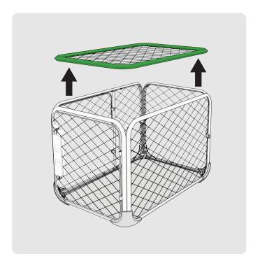
Flip your crate over so the open base panel is facing upward. For the Intermediate and Large crate sizes we recommend 2 people flip the crate.
