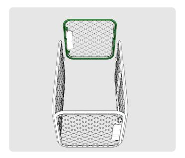
Re-install the open base panel and its four (4) base corner connectors. Make sure that the feet are oriented upwards.
