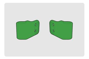
Screw these edge connectors into the new door panel in the orientation shown below. Be sure to pay extra attention to both the orientation of the connectors and the orientation of the panel.
