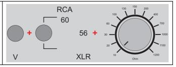
Alternative setting with with fixed input impedance. Setting for Low-Output MC cartridges with a recommended input impedance of  $\leq 10$  Ohm.
