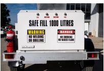
connection points. These suction and connection points are conveniently located at the rear of the trailer for simple / quick connection to site equipment. We provide foot valves on the 2 x suction points to ensure that you retain a prime on the suction line to your generator, lighting tower, compressor or pump.
