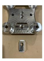
Remove the radius rods, pull plate and slide the bulkhead bracket over the factory studs. Then mark the 6 mounting holes with a marker or center punch.
