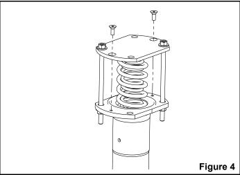
9. Slowly draw the cover down onto the spring box by alternately tightening each rod.
