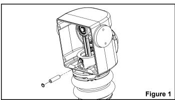
7. Remove the six hex head flange screws (page 16, #21) holding the spring box guard (page 16, #12) to the bottom bellows ring (page 16, #4).
