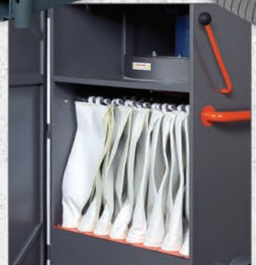
Long-Lasting Polyester Filters with Manual Shaker Handle
