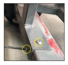
Secure hose minder to bottom of the saw frame with the 4 - 7/16<sup>th</sup> self-tapping screws (provided).
