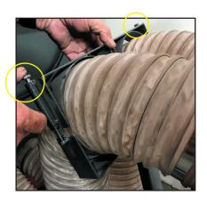
Place hose minder top piece over hoses and reattach to bottom piece with the original side bolts.
