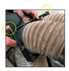
Remove top piece from hose minder attachment by loosening the 2 side bolts with ratchet.
