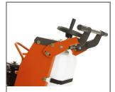
**ADJUSTABLE HANDLES**Provides a closer and more comfortable position to the cutting side for easier alignment and straighter cuts. Handle can also be folded for transport.
