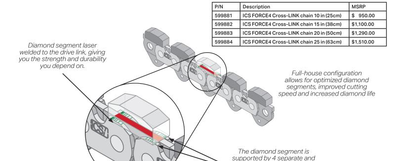
Drive Links, Tie Straps and Segments work in concert to prevent reverse articulation and increase stability in the cut, providing a smoother cutting experience with less operator effort
