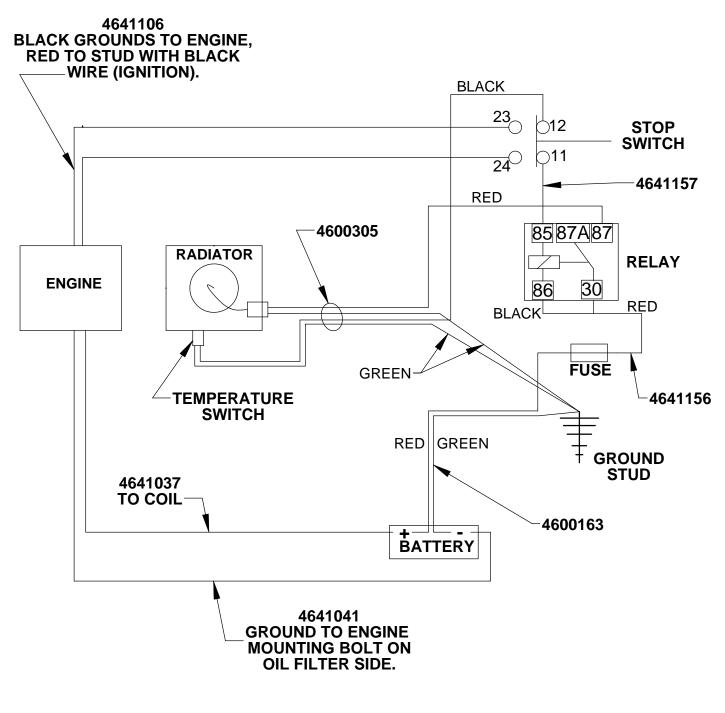
WIRES ARE IN KIT 4640125 (DOES NOT INCLUDE BATTERY CABLES)
