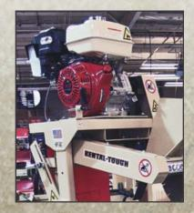
EDCO's fixed engine isolates the power source from the cutting arm, reducing blade vibration, and eliminates lowoil situations that cause engine burnout.
