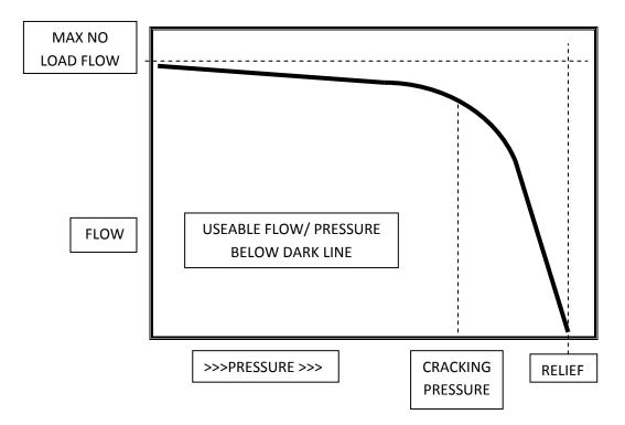
Flow decreases as engine/motor RPM drops under load. Relief valves begin to open and shunt flow to tank at 75-80% of the relief setting (cracking pressure). This further reduces flow to the tool. At relief, all flow is directed to tank.
