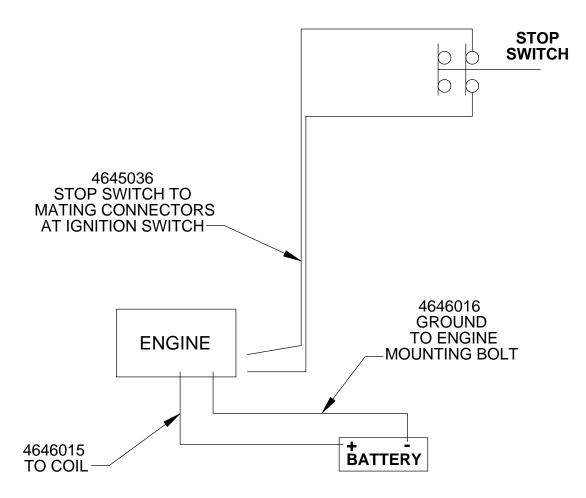
FOR EASE OF ASSEMBLY, ATTACH WIRES TO STOP SWITCH BEFORE INSTALLING IN PANEL.
