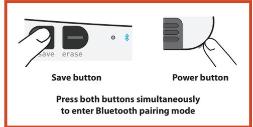
To disable Bluetooth connectivity: Turn off the Boogie Board Sync eWriter, and then press the **ERASE** button while simultaneously pressing the **POWER** button. Bluetooth may need to be disabled on airplanes and other environments (e.g., hospitals).
