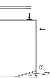
1. End of the stylus attaches to the four metal plates around the sides of the product.
