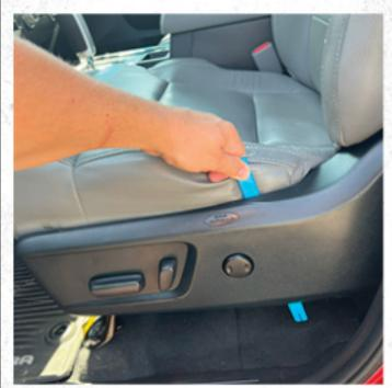
In Toyota Tundra trucks the Paracord Seat Cinch™ should be routed between the outside of the seat cushions and the inside of the plastic trim panels around the outside of the driver and passenger seats (where the seat controls are located).
