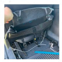
Feed both ends of the paracord down around the bottom of the seat cushion. Then
