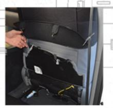
These bungees will remain disconnected and the flap will be folded up and inside-of the new seat covers later in the process. You must disconnect this flap in order to properly install the new seat covers.
