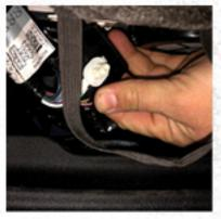
Unhook the connector from the frame, then remove the elastic that is wrapped around it. Then reconnect the plastic connector to the seat frame.
