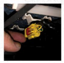
Pull down (or twist slightly) on the plastic electrical connector (gray/yellow) that the bungee is wrapped around.
