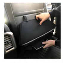
Next, working from behind the seat, tuck the original carpet flap (that was disconnected in step #2 above) up and inside of the new seat cover. It will fold flat against the pocket of the seat.
