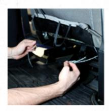
Feed both ends of the paracord down around the bottom of the seat cushion. Then locate both ends underneath the back-side of the seat and adjust the positioning of the knot by pulling the entire paracord through the sleeve to one side or the other, as needed. Then connect them together with a simple loop and temporary knot underneath the backside of the seat.
