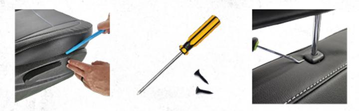
Vehicle's equipped with the 40-20-40 front bench seats will require a screwdriver to remove the (2x) screws in the bottom of the front cup holders. The 2019 to current models will also have (2x) screws in the integrated seat belt molding attached to the front-driver's side of the folding center console.
