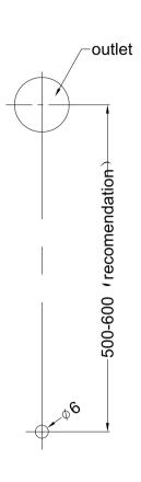
1.Drill a φ6mm hole at the downwards outlet vertical downward position in the recomendation range.
