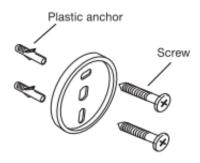
3. Mount the holder to the wall using the screws and the plastic anchors provided. Take care to mount vertically even.
