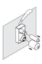
5 Install the flange and handle. It is recommended to apply a small bead of silicone behind the faceplate to prevent water entering the wall cavity.
