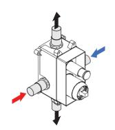
3. Fasten the mixer body to the wall, ensuring that it is level.
