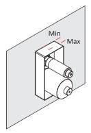
2. Connect the hot and cold water inlet pipes and the outlet pipe.
