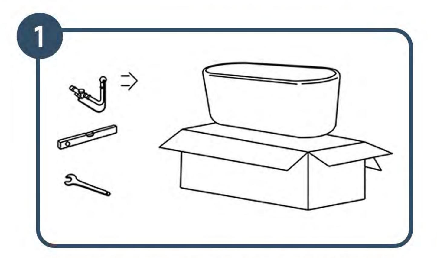
Remove your freestanding bath from the packaging & place it in the correct location for installation. Check for damage & ensure your freestanding bath is kept away from any rubble, rough surfaces or heavy objects during installation.
