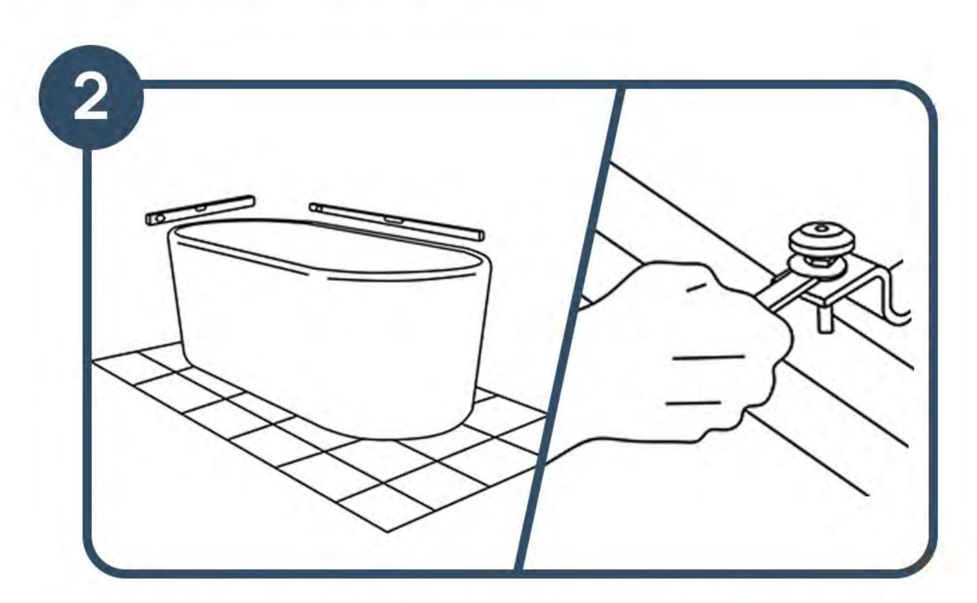
Adjust the self-levelling feet so that the base is level and 1 – 5 mm above the finished floor. Use a spirit level to ensure the bath is level to allow all water to drain away smoothly to the waste outlet.
