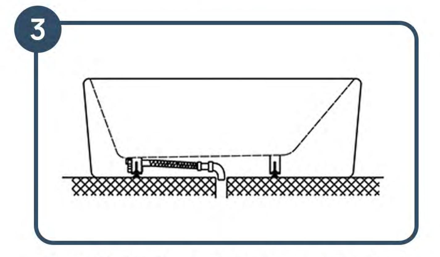
Carefully tilt the bath to connect the drain pipe to the outlet. We recommend using a flexible connector.
