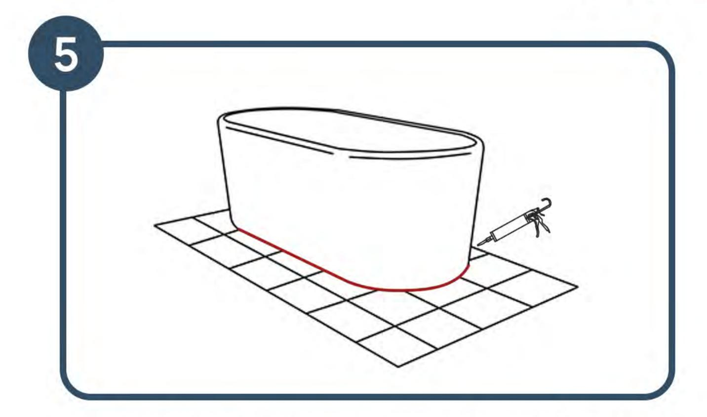
Apply silicon around the base of the bath to prevent movement. Allow to set for 24 hours.
