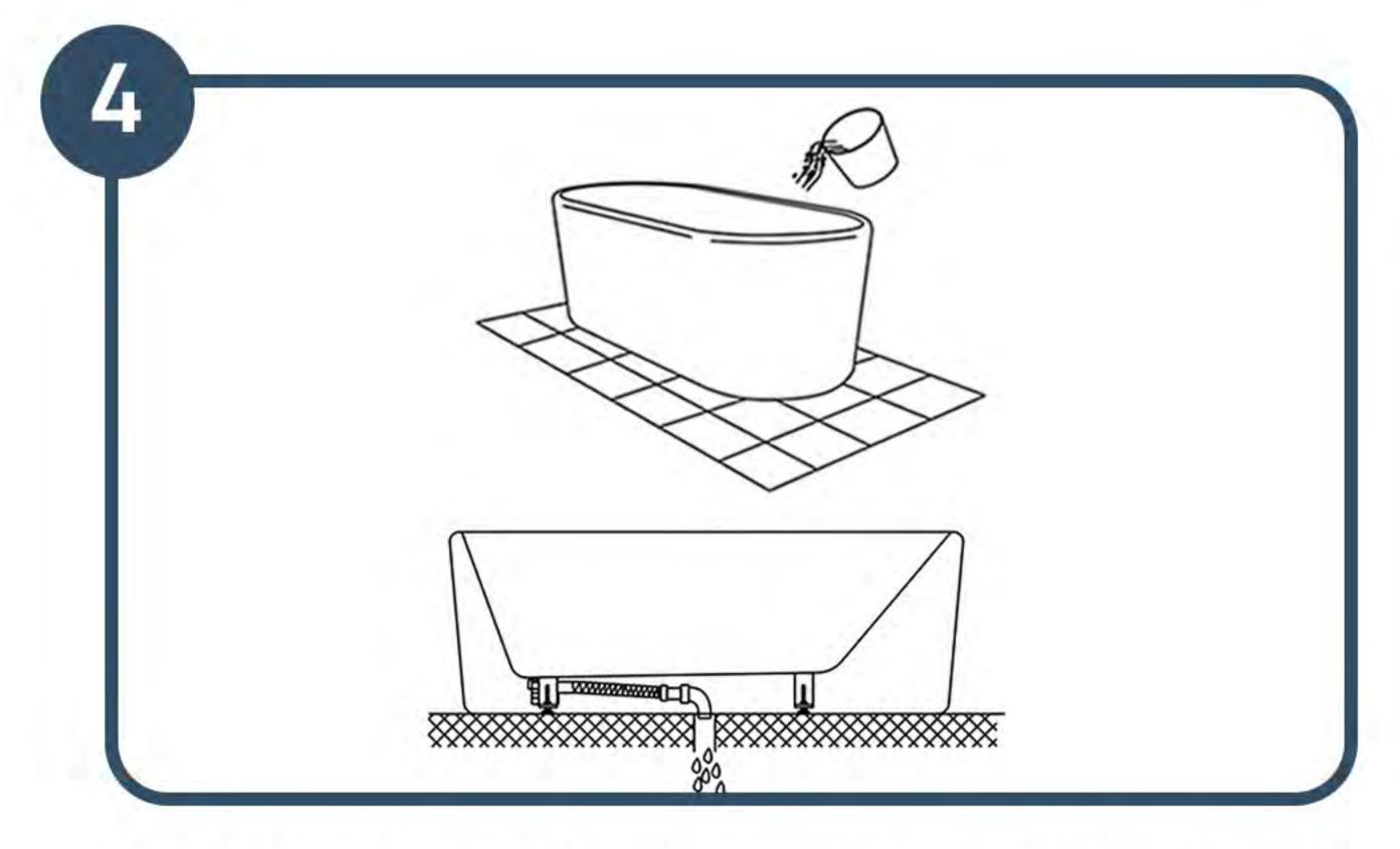
Before sealing in place, check the bath for leaks and correct drainage by filling the bath with water and ensuring water flows easily through the waste outlet.
