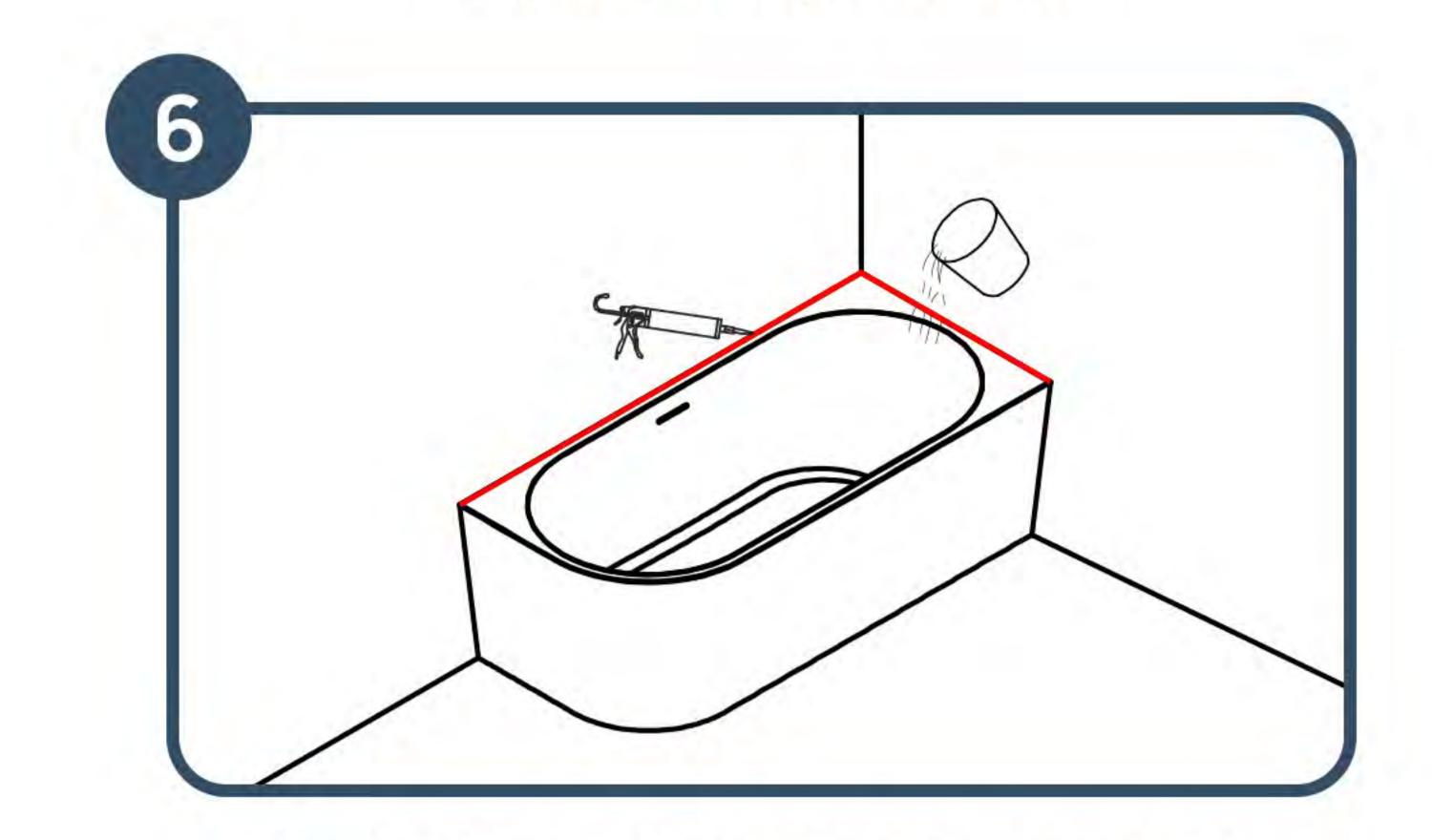
Before sealing in place, check the bath for leaks and correct drainage by filling the bath with water and ensuring water flows easily through the waste outlet. Apply silicon along the back and side edge, against the wall and around the base of the bath to prevent movement. Allow to set for 24 hours.
