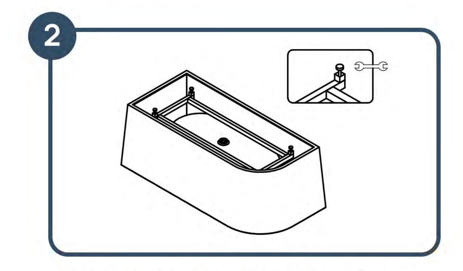
Remove your corner bath from the packaging & place it in the correct location for installation. Check for damage & ensure your corner bath is kept away from any rubble, rough surfaces or heavy objects during installation. Adjust the self-levelling feet so that the base is level and 3 – 5mm above the finished floor. Use a spirit level to ensure the bath is level to allow all water to drain away smoothly to the waste outlet.
