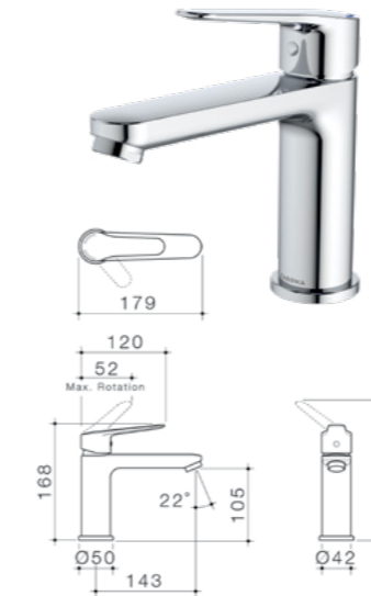
Opal Basin Mixer H/C WELS 6 star rated, 4.5L/min ● 99700C6A ● 99700B6A ● 99700BN6A
