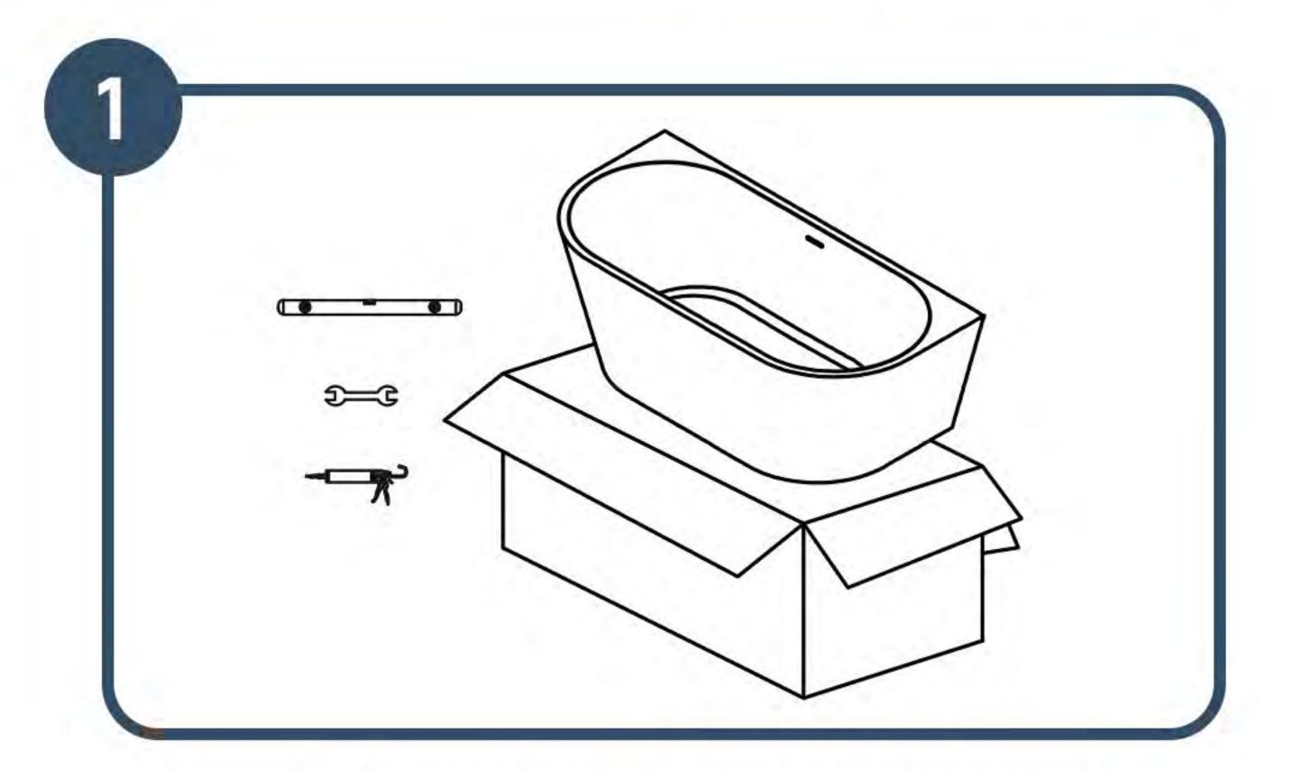
Remove your back to wall bath from the packaging & place it in the correct location for installation. Check for damage & ensure your back to wall bath is kept away from any rubble, rough surfaces or heavy objects during installation.
