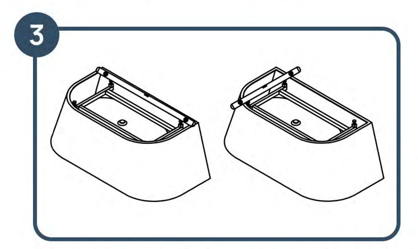
Carefully tilt the bath to connect the drain pipe to the outlet. We recommend using a flexible connector.
