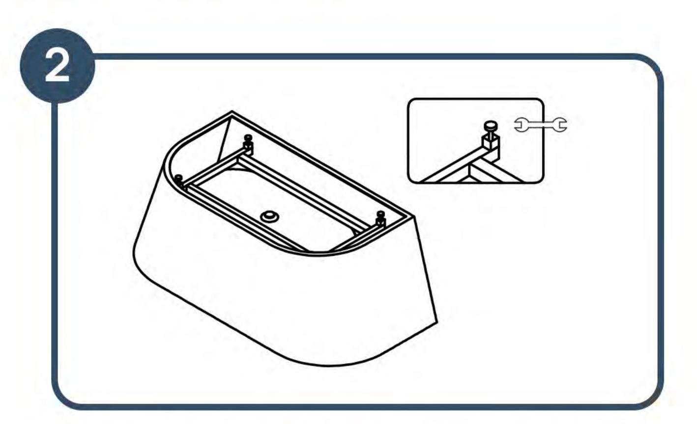
Adjust the self-levelling feet so that the base is level and 3 – 5mm above the finished floor. Use a spirit level to ensure the bath is level to allow all water to drain away smoothly to the waste outlet.
