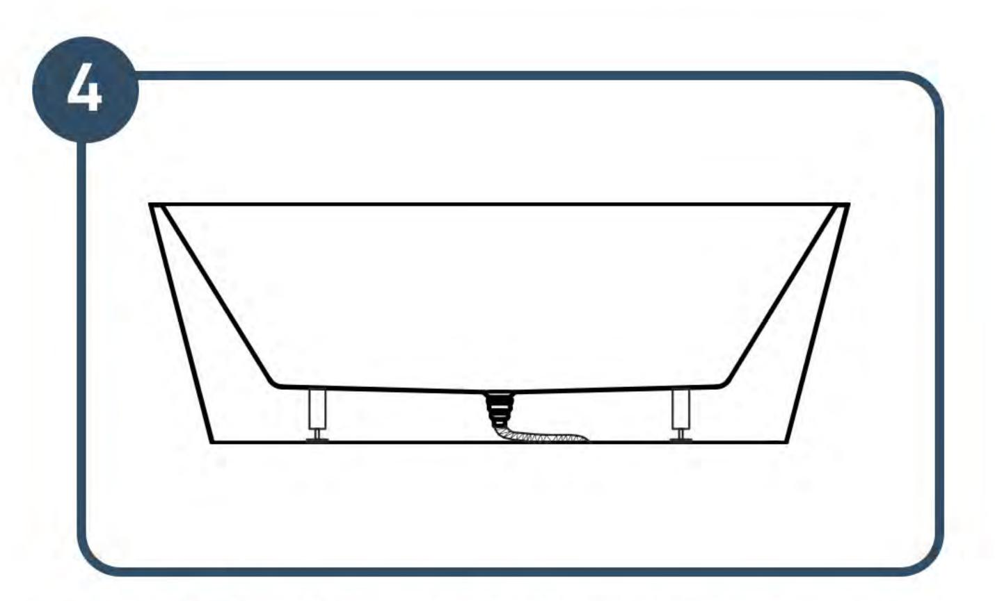
Carefully adjust the bath against the wall to the correct installation position, check and adjust with spirit level.
