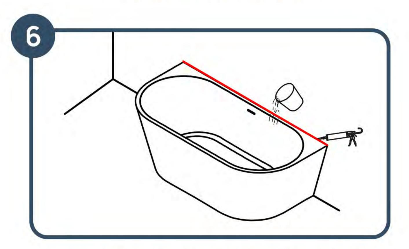
Apply silicon along the back edge and around the base of the bath to prevent movement. Allow to set for 24 hours.
