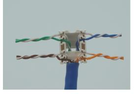
Verify conductors are seated according to T568A or T568B code.
