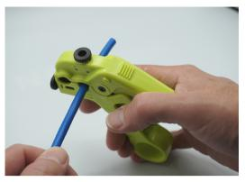
Remove 2" of cable jacket, carefully avoid nicking any conductor.
