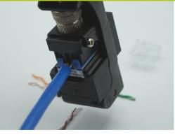
Close tool handle to seat **O** & flush cut conductors.
