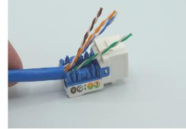
Line up pairs to seat according to T568A or T568B sequence.
