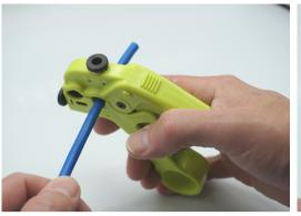
Remove 2" of cable jacket, carefully to avoid nicking a conductor.
