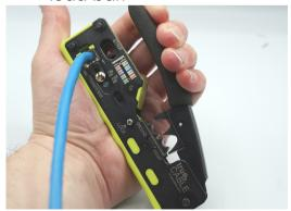
Place entire assembly into crimp tool. Fully close handle to complete crimp process.
