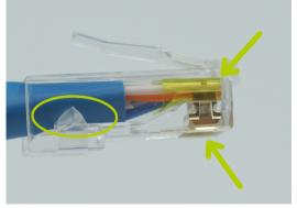
Inspect. Load bar fully seated, all golden contacts seated, strain latch engaged.
