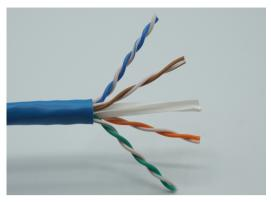
Remove 1.5" of cable jacket. Separate conductor pairs. Remove spline & untwist pairs.
