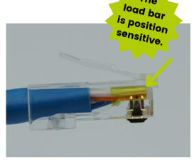
Insert load bar/cable assembly into RJ45 plug housing. Seat until load bar stops at front.
