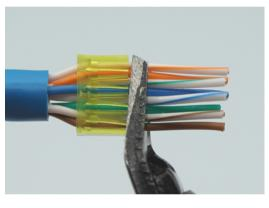
Seat load bar no further than 1/4" from end of cable jacket. Flush cut at front of load bar.
