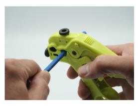
Remove 2.5" of cable jacket, carefully avoid nicking any conductors. Do NOT remove foil shield.
