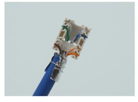
Carefully flush cut conductors from sides of termination cap.
