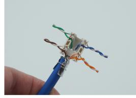
Insert conductors into either T568A or T568B color sequence.
