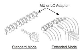
Insert tip of cleaner into MU/LC Adapter.
