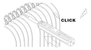
Push the Outer Shell to start cleaning the MU/LC connector end face. A "click" sound indicates end of cleaning process. Close the dust cover after use.
