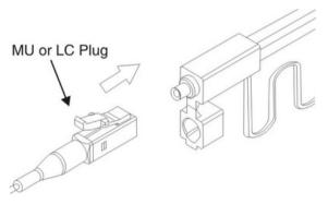
Insert MU/LC connector into the Guide Cap.
