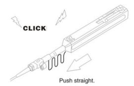
Push the Outer Shell to start cleaning the MU/LC connector end face. A "click" sound indicates end of cleaning process. Close the dust cover after use.
