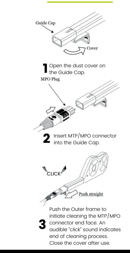
Push the Outer frame to initiate cleaning the MTP/MPO connector end face. An audible "click" sound indicates end of cleaning process. Close the cover after use.
