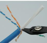
Remove ripcord, any PE tape or waterproof tape, and then remove spline.
