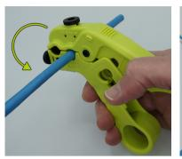
Strip 2" of cable jacket from cable. Be careful not to nick conductors!
