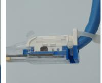
2 For Position #3, use the optional nylon tie as shown. This provides an upward cable angle.
