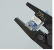
Parallel jaw pliers in use. Cat6A cable will often require pliers. Use inside steps on trueCABLE brand pliers, placing the plug as to apply even pressure on the plug housing.
