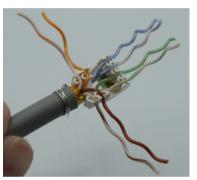
6 Untwist conductors and seat according to either T568A/B sequence. Keep untwist to ½" or less. T568B shown.
