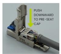
Insert cap into housing. It fits one way, aligning on the white notch. Press cap down to pre-seat before closing lid!
