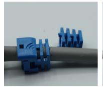
Cut the locking strain relief boot to fit the cable jacket. Slide boot down out of the way.
