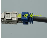
Slide locking strain relief boot over rear of housing to lock closed. Match the WiFi symbols up.
