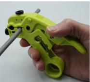
2 Strip off 3" or more of cable jacket. Strip off enough jacket for excess ESD drain wire to wrap around cable jacket.
