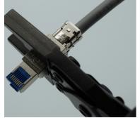
Close with parallel pliers or channel locks. Close hinged lid by placing pressure at middle of housing.
