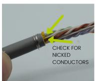
3 Remove shield & other wraps. Wrap ESD wire around cable jacket no further than <sup>3</sup>/<sub>8</sub>" back.
